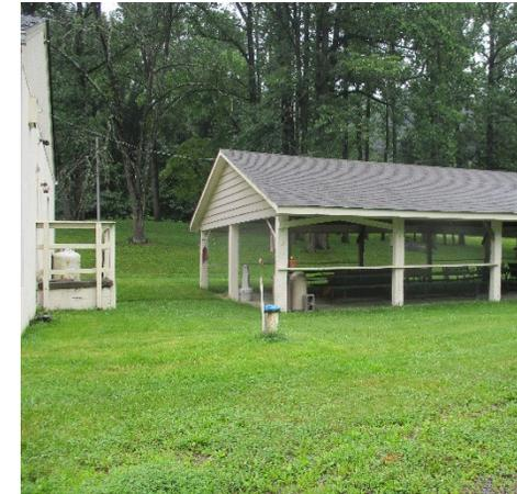
A rain garden can be installed east of the building near a disconnected downspout to capture, treat, and infiltrate rooftop runoff. A preliminary soil assessment suggests that more soil testing would be required before determining the soil's suitability for green infrastructure.
